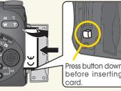
Insert the memory card with the Nikon CompactFlash™ label facing the front of the camera (the side with the lens). Make sure to insert the edge with the contact points (two rows of small holes) into the camera.
