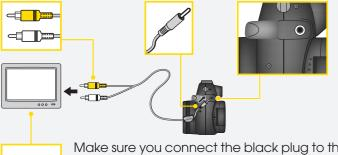
Make sure you connect the black plug to the camera, and the yellow plug to the television Video-in socket, and the white plug to the television Audio-
